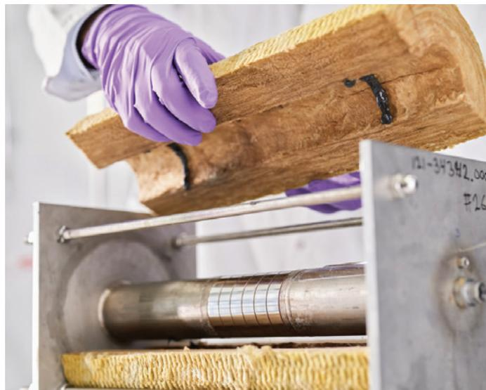
A technician prepares an ASTM G189 test cell by applying a section of ProRox® PS 965 with CR-Tech™ around a pipe section containing carbon steel coupons. ASTM G189 is the standard guide for laboratory simulation of CUI. This test can be used to simulate an accelerated corrosion environment to compare corrosion rates of different combinations of insulation systems.
