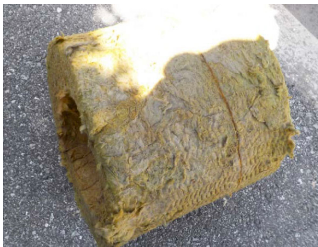
Figure 3. After three years at 120 – 140 °C (248 – 284 °F), the ProRox PS 960 with WR-Tech maintained its structural integrity and showed minimal ingress of water.
