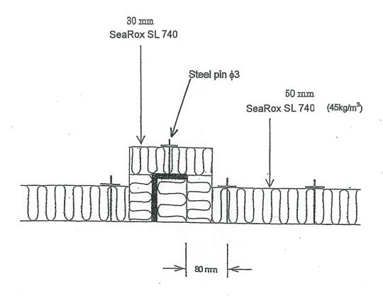
Diameter of washer: 30mm or 38mm
