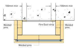
$\textbf{Figure 10} \ \ \textbf{Three-sided protection for rectangular ducts, using welded} \\ \textbf{pin fixing method}$
