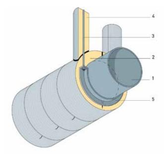
Figure 1 Fire Duct Section applied to circular duct
