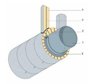
Figure 2 Fire Duct PSM applied to circular duct
